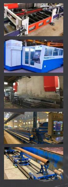
Laser cutting machine Bystronic Bystar 4025 Width up to 2500mm Lenght up to 6500mm Power 6kW
